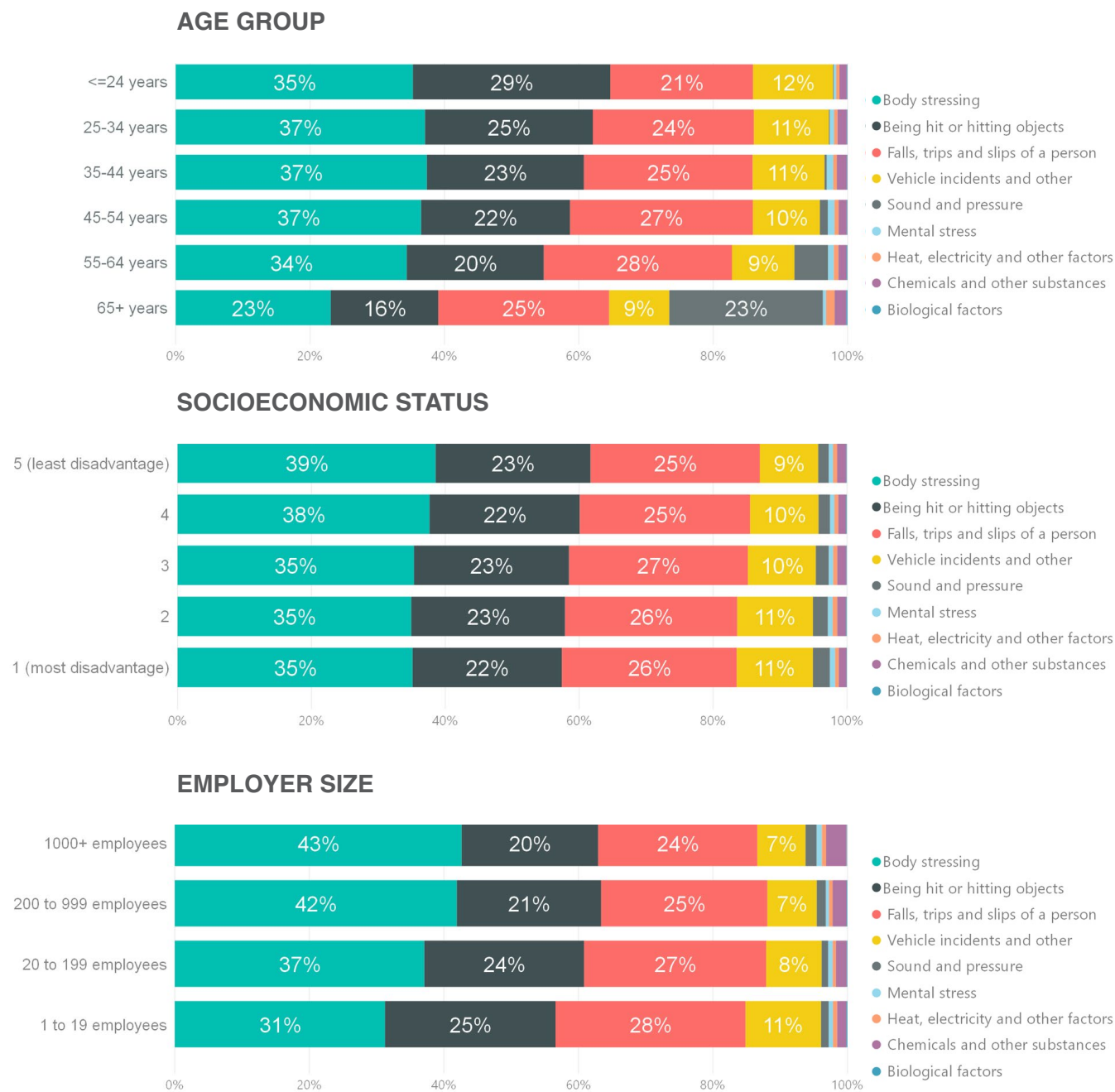
Figure 7 Mechanism of injury by age, socioeconomic status and employer size groups in truck drivers
